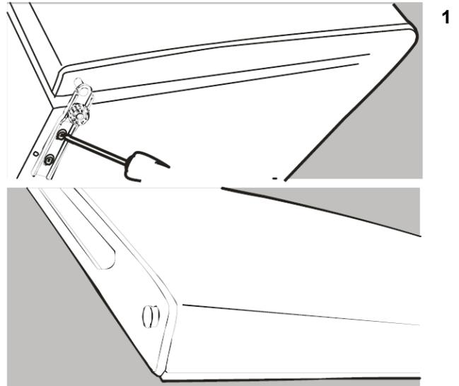
2. Remove the top hinge cover from door first. Then unscrew the two screws from top door hinge and replace on the other side.
