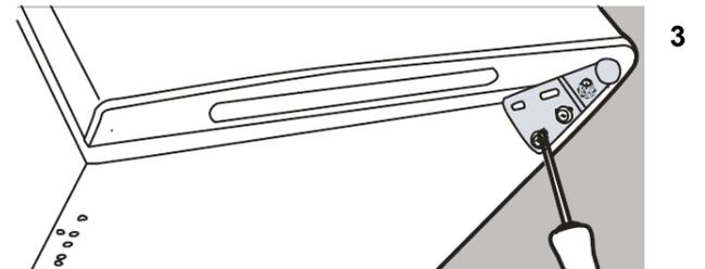
4. Screw the bottom hinge into place on the new side. Replace the leg on the other side.
