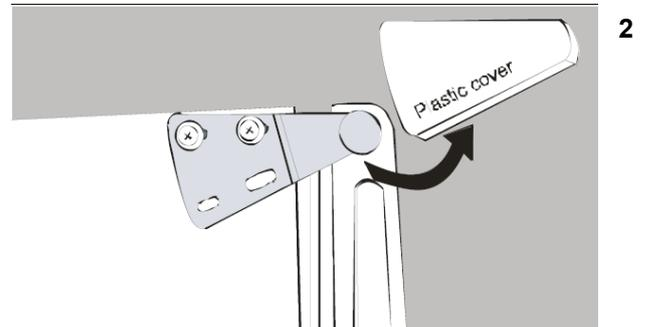
3. To install the top hinge on the left side of the appliance, secure the two screws through the hinge and into the top of the appliance. Slide the door back on to the top hinge. Ensure the door is face up. Replace the top hinge cover on the top hinge by pressing down until it clicks into position.
